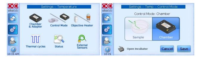
The system may ask you if you want to calibrate. Please know that it takes several hours. It is not necessary if the room temperature is within 1C from 23C. If the room temperature differs by more than 1C from 23C you can calibrate OR you can operate in sample feedback mode. Select 'Sample' and make sure to insert the green thermocouple into a reference well. Ensure that the tip of the thermocouple is fully immersed in liquid. You can use tape to hold the thermocouple in place.
